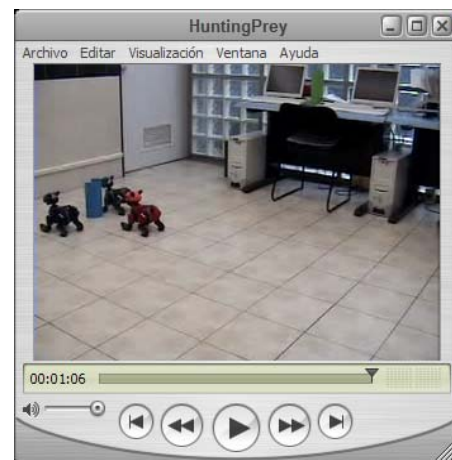
Fig. 14. Hunting model with one prey, an alpha wolf and two beta wolves. Beta wolves move ahead of the pack to attack prey.
