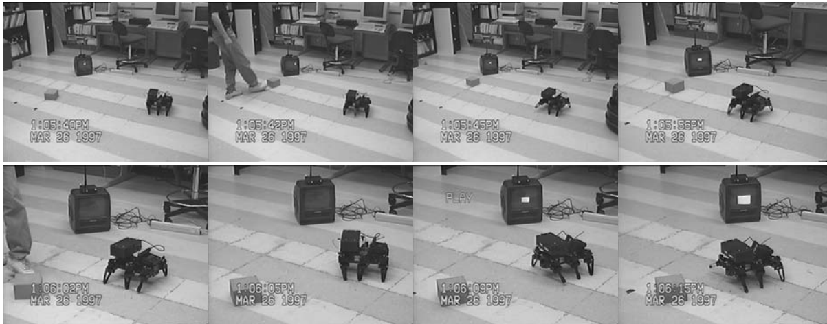
Fig. 15. This sequence of pictures shows Miguel following a prey as it is moved around. The sequence proceeds from left to right. The prey is represented by an orange box. The video monitor shows the broadcast results of Miguel's visual processing. Note how in the bottom two photographs the region size increases as Miguel approaches the prey object.
