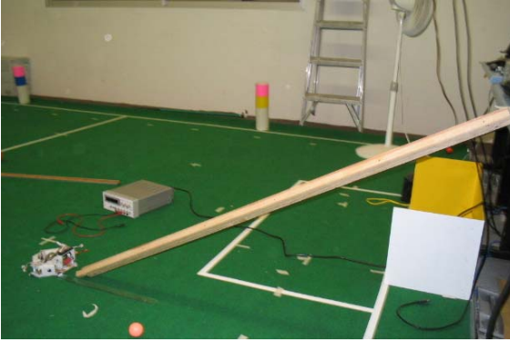
Fig. 12. Dribbler prototype consisting of a launch pad where the ball is manually dropped. The launch pad directs the ball into the robot dribbler.
