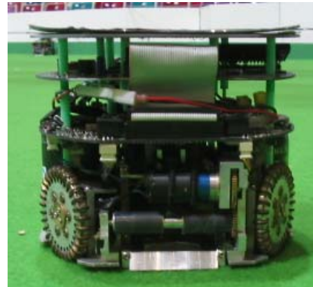
Fig. 9. Fu-Fighters SSL Robot. The dribbler includes a separation in the middle of the bar to center the ball.
