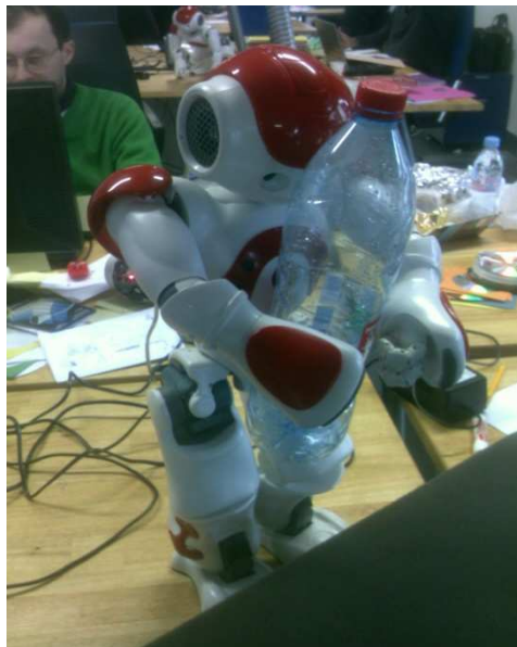
Fig. 1. The Aldebaran Nao. In this image, a spoken language command processed by RAD and sent over the internet was issued to activate a pre-recorded Choregraphe script for grasping an object and then standing up in preparation to carry the object to the user. This will contribute to the fetch and carry task.
