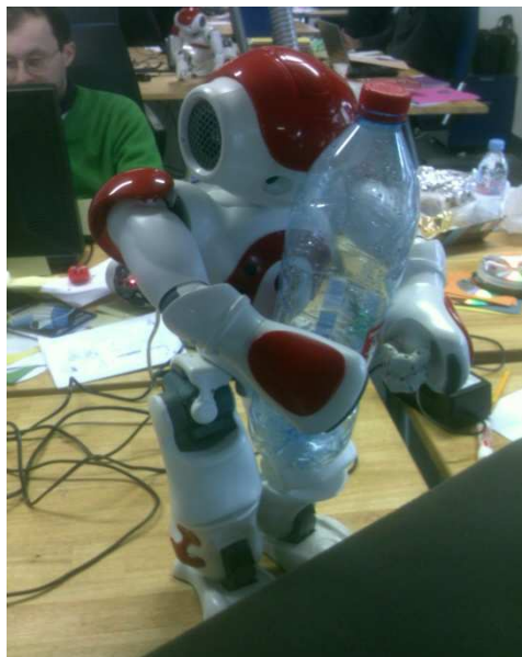
Fig. 1. The Aldebaran Nao. In this image, a spoken language command processed by RAD and sent over the internet was issued to activate a pre-recorded Choregraphe script for grasping an object and then standing up in preparation to carry the object to the user. This will contribute to the fetch and carry task.
