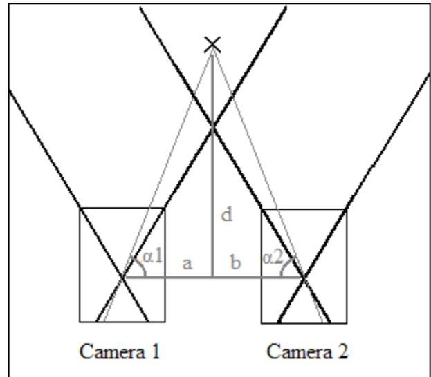
**Fig. 2: Stereo vision object distance computation**
