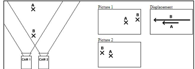
**Fig. 1: Stereo vision with two parallel cameras**
