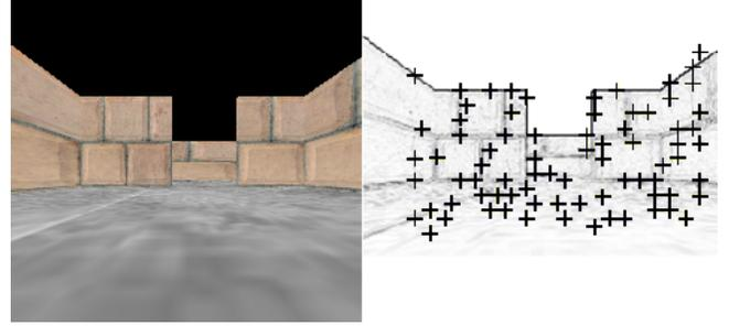
**Fig. 6: Relevant points calculation (from the left contrasts picture)**
