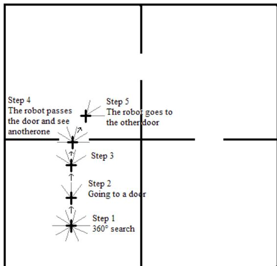
**Fig. 12: The diagram shows intermediate steps as the robot goes from a room to another one**
