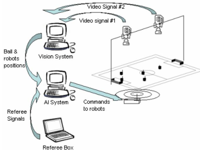
Fig. 1. Typical architecture of a SSL team
